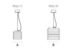
The collection originally designed by Tapiovaara in 1955 now incorporates LED technology, capable of blending functionality and intimacy at the same time, and it has been re-edited in two sizes, with fifteen- or thirty-centimetre diameter discs. With both models, an inner white glass diffuser helps to filter the light.
