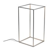
Floor lamp providing diffused light. Extruded aluminium frame 10x10x1 gratiné and anodized in various finishes. Led on the top edges incorporated in the extrusions and protected by transparent PC diffusers. Driver on plug, dimmable switch on chord.
