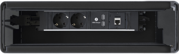
IN USB Charge · 2 safety plugs and 1 USB dual charger · 1 module for flexible use (here: RJ45 CAT6) · Power input: GST18; Power output: GST18 · Cable length: 3 m · Aluminium panelling
