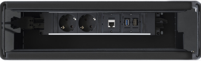
IN Free · 2 safety plugs · 2 two modules for flexible use (here: 1 Slot USB 3.0, HDMI 2.0 And RJ45 CAT6) · Power input: GST18; Power output: GST18 · Cable length: 3 m · Aluminium panelling
