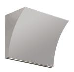
Wall lamp providing direct/indirect light. Pressure die-cast Zamak alloy structure, matte gray, shiny white or chrome plated finish. Molded steel, galvanized white wall attachment containing the wall attachment system as well as the electrical devices.
